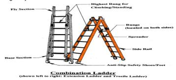
A Combination Ladder is a portable ladder. This type of ladder can be designed with either steps or rungs, and the inclusion of a pail shelf is optional. When steps are present, the ladder should be erected so that the step surfaces are horizontal. Either spreaders or a locking device can be used to securely hold the front and rear sections in the open position.
