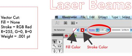
To score into a material, vector lines must be RGB **Blue**, **Green**, Yellow, Magenta, Cyan or Orange. You can use the different colors to set up variations in cut depths within an image. The power and speed settings for each color will be executed in the Universal Laser Systems Control Panel (UCP) program.
