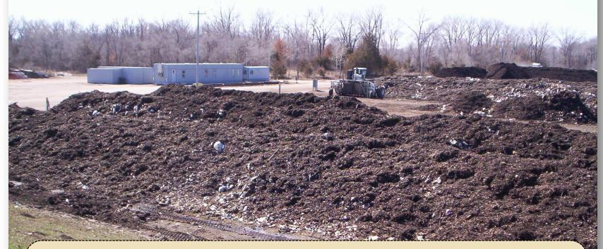
Complete piles are covered with a natural bio-filter of leaves and compost. Active piles will reach and maintain a temperature of at least 131 F. After meeting the Process to Further Reduce Pathogen (PFRP) requirements, piles will be moved to a curing area.
