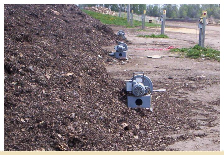
Blowers cycle on and off to keep adequate oxygen levels in piles and maintain an aerobic environment.
