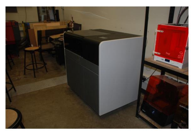
The Projet MJP 2500 prints in clear resin with a wax based support structure.
