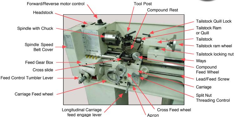
12" Gap Bed Gear Head Lathe
